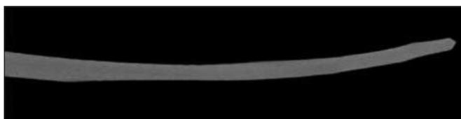
**Figure 2:** File scanned image after use showed visible defects, combined defects (unwinding and curving).
