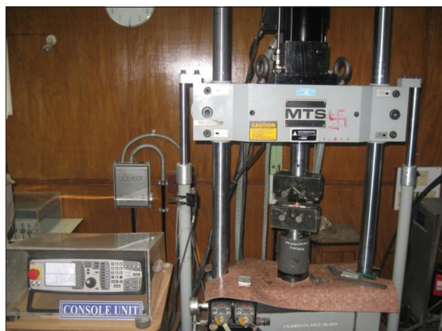
Figure 6: The block with embedded root were mounted on to the loading frame of material testing system.
