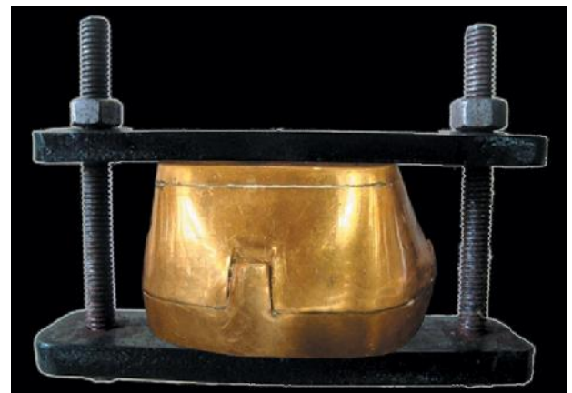
Figure 8: R.S. Tension Plate Assembly with Flask.
