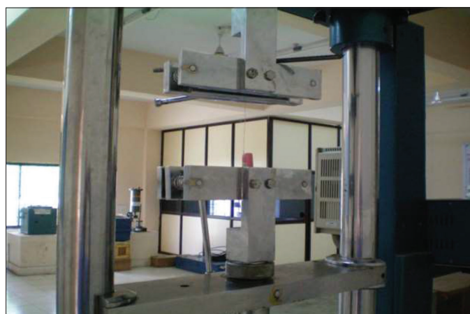
Figure 3: Shearing of composite material using universal strength testing machine.
