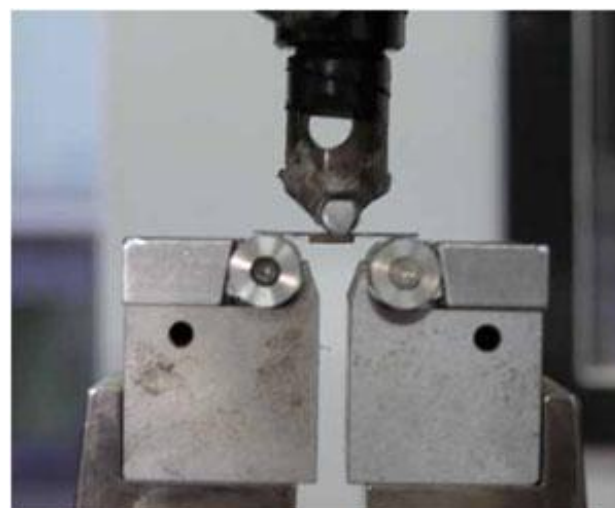
Fig. 3: Three-point bending test on a Universal testing machine.
