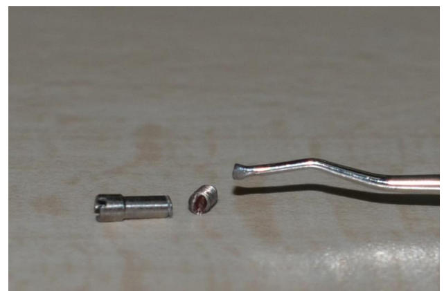
Fig. 2: Retrieved fractured abutment screw and the modified end of the spoon excavator used for the procedure.
