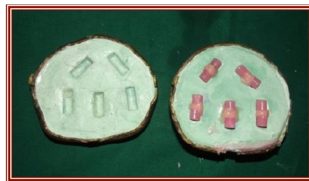
Figure 3: 4 mm section of PMMA cylinders packed with the test material.
