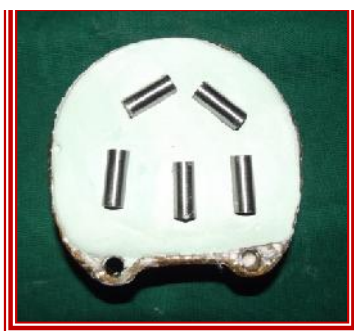
Figure 1: Flashed Aluminium cylinders and heat cured PMMA Cylinders.
