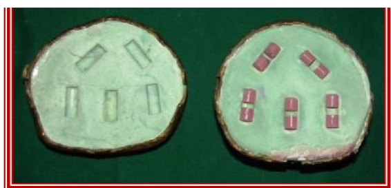
Figure 2: 4 mm sectioned PMMA specimens.
