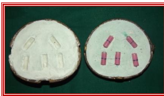
Figure 1: Flashed Aluminium cylinders and heat cured PMMA Cylinders.
