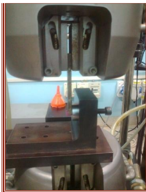
Figure 4: Tensile and Shear bond strength testing of the specimens.
