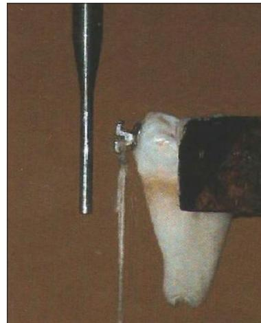
Figure 1: Acrylic mounted for the shear test.
