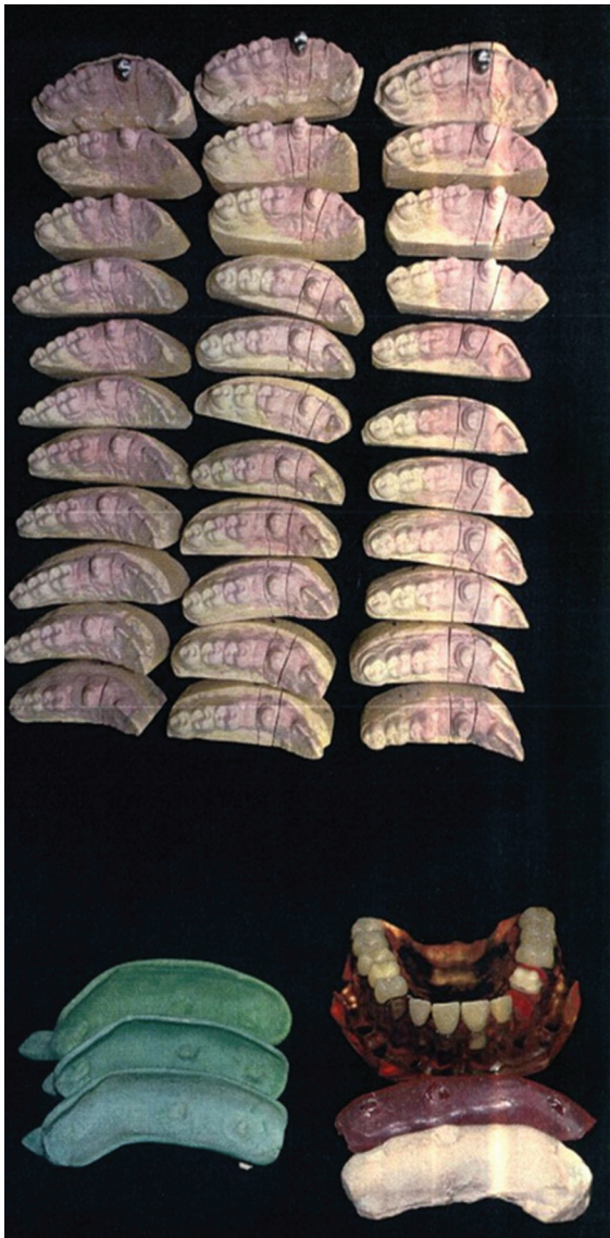
Figure 1: Duplicated dies which were prepared by three types of impression materials (Speedex, Panasil, and Impergum).
