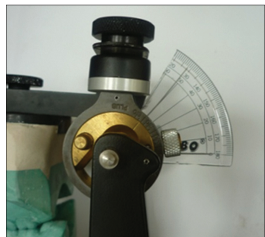
Figure 1: Modification of Hanau articulator using template protractor.
