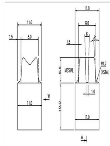
**Figure 1:** Schematic representation for computer aided designing design of zirconia die.
