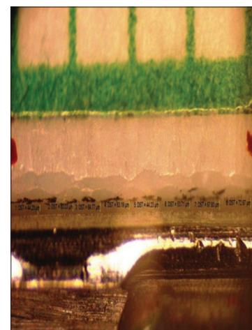
**Figure 5:** Stereomicroscopic photograph of a specimen of Group-3a (metal copings) while measuring the marginal gap.
