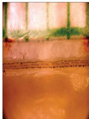
**Figure 3:** Stereomicroscopic photograph of a specimen of Group-2a (zirconia copings) while measuring the marginal gap.
