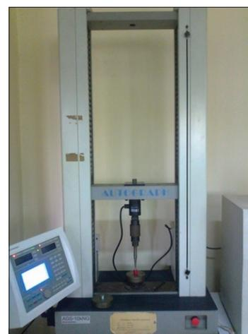
**Figure 4:** Measuring fracture strength by using universal testing machine.
