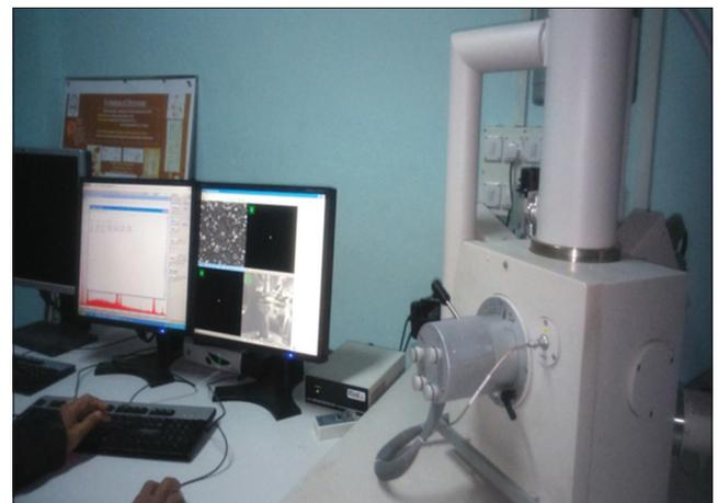
**Figure 1:** Scanning electron microscope (E-SEM – Quanta200, The Netherlands).
