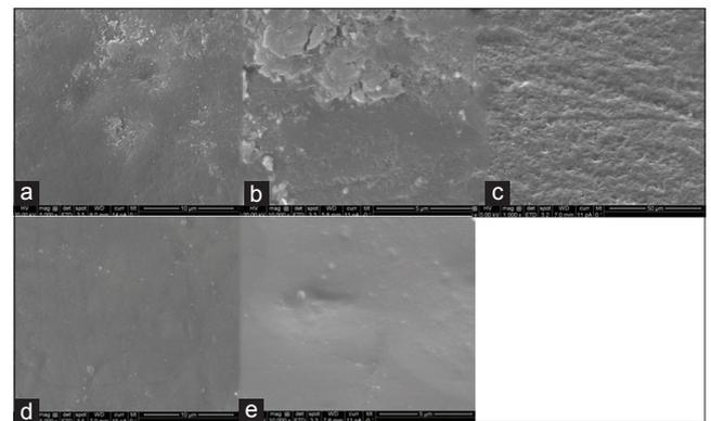
**Figure 3:** Scanning electron microscope results: (a) Baseline, (b) demineralized, (c) after 7 days brushing, (d) after 14 days brushing, (e) after 21 days brushing.
