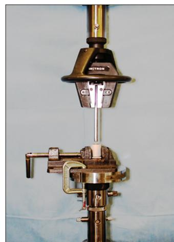
Figure 1: The specimen loaded in Instron machine for testing.
