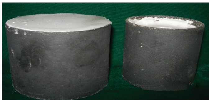
Figure 16: Investing of the wax patterns.
