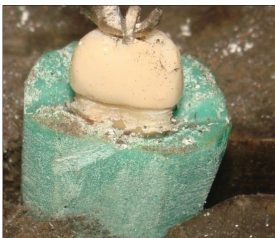
Figure 5: Crown pull test.
